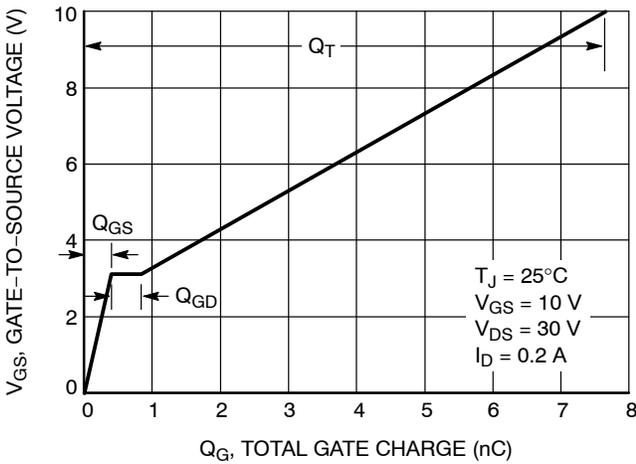
Figure 5. Gate-to-Source and Drain-to-Source Voltage vs. Total Charge
