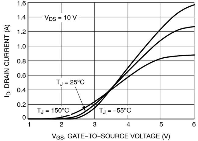
Figure 2. Transfer Characteristics
