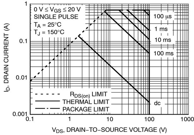
**Figure 7. Maximum Rated Forward Biased Safe Operating Area**
