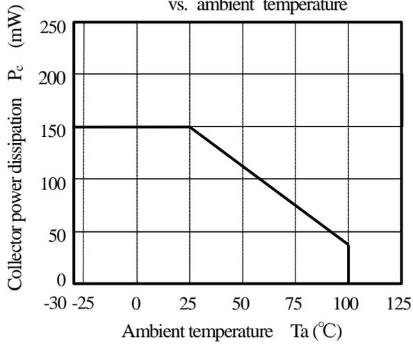
(Fig. 4) Total power dissipation vs. ambient temperature
