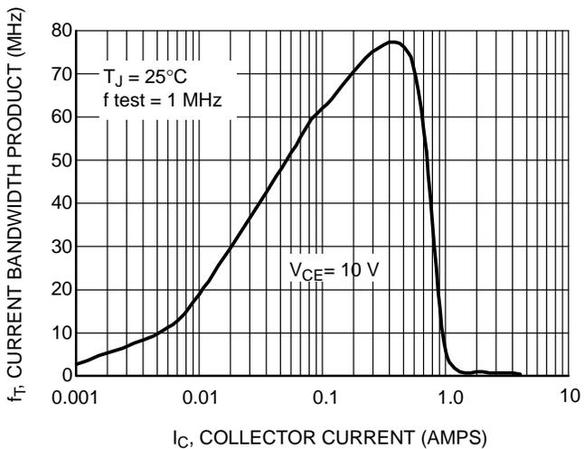
**Figure 14. Typical Current Gain Bandwidth Product
