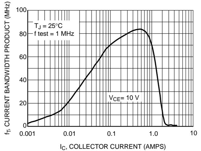
**Figure 15. Typical Current Gain Bandwidth Product
