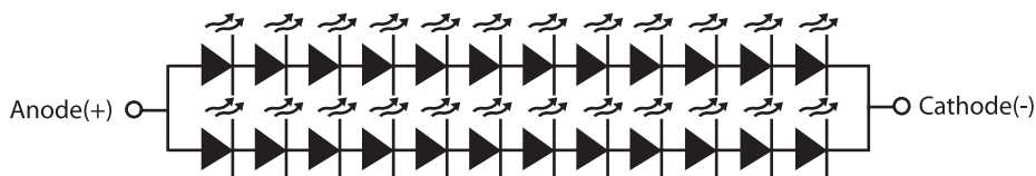
9W EdiPower® II HM Series Circuit Layout
