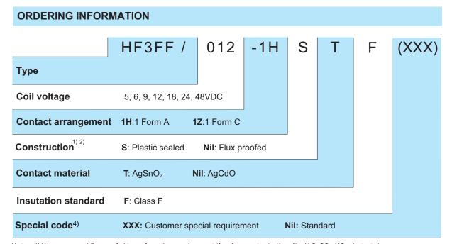
Notes: 1) We recommend flux proofed types for a clean environment (free from contaminations like H<sub>2</sub>S, SO<sub>2</sub>, NO<sub>2</sub>, dust, etc.).
