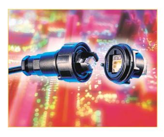
Shroud for RJ45 provides protection against damage Coupling ring, screw thread provides secure cable coupling through mis-use and positive alignment for mating of connectors Panel gasket maintains IP68 seal to panel Sealing gland and cage optimised to maintain IP68 seal and provide secure cable restraint without disrupting signal 'O' ring maintains IP68 seal Shielded Cat 5e coupler at connector interface maintains screening
