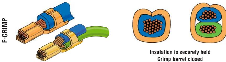
For double wire applications with different size wires always place wire with smallest outer diameter in the bottom
