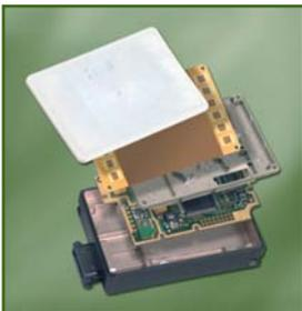
Tyco Electronics is a world leading supplier of radar technology for the automotive industries. In cooperation with system integrators and OEMs, Tyco Electronics developed 24 GHz high resolution short range radar sensors in Ultra Wide Band technology and 77 GHz Adaptive Cruise Control radar front ends suitable for driver assistance applications, which enable advanced active and passive safety systems.
