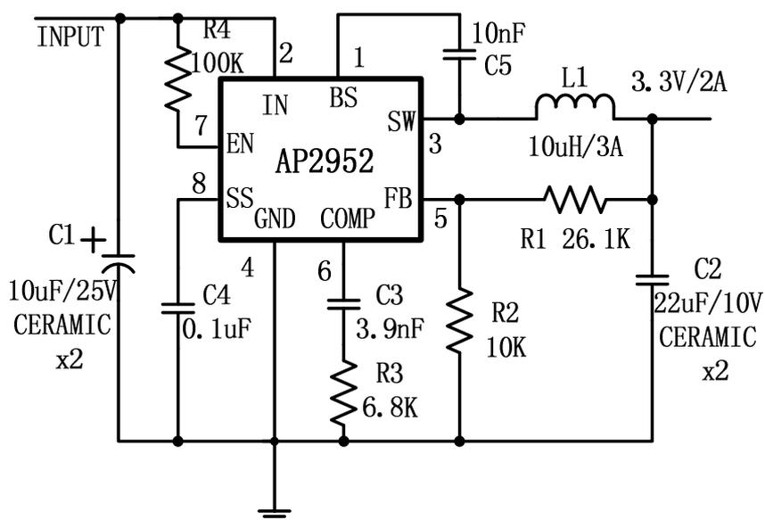
Figure 5 AP2952 with 3.3V output, 2X22uF Ceramic Output Capacitor
