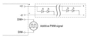
"DO NOT connect "DIM- to -V"
