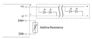
"DO NOT connect "DIM- to -V"
