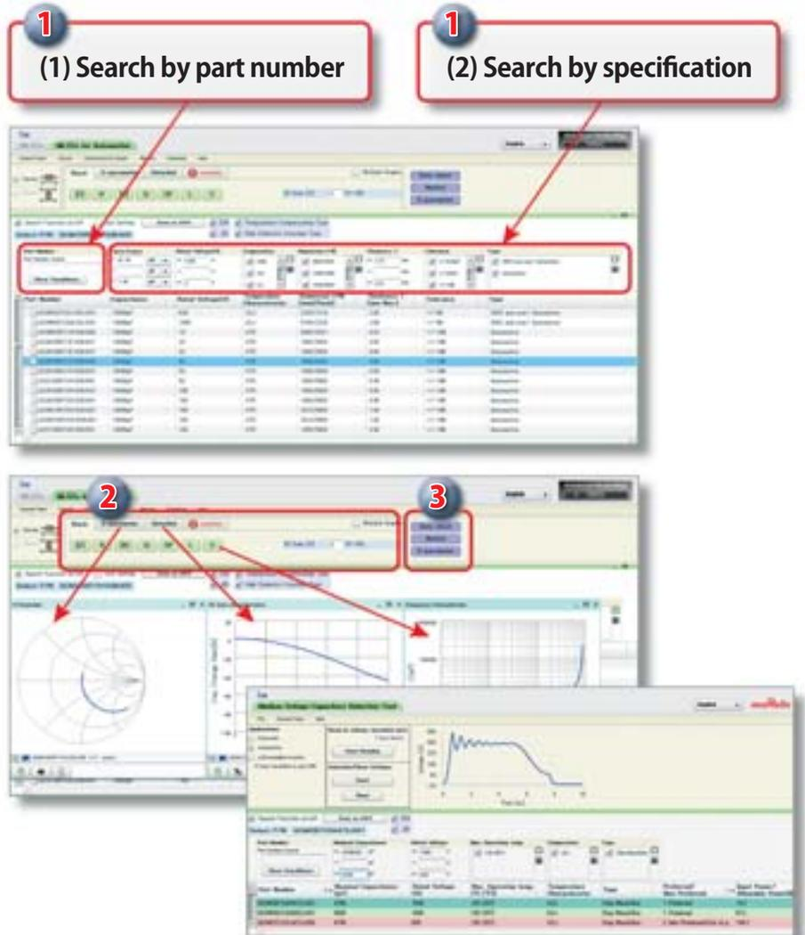
The image shows three sequential screenshots of the SimSurfing MLCC tool interface. The first screenshot shows a search interface with two options: (1) Search by part number and (2) Search by specification. The second screenshot shows a list of search results with columns for part number, capacitance, and other parameters. The third screenshot shows a detailed view of a selected part, including a frequency response chart and a table of electrical characteristics.
