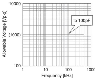
The sine-wave frequency VS allowable voltage
