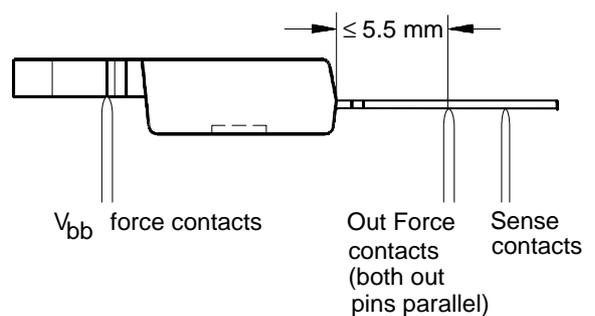
23) Low ohmic short to  $V_{bb}$  may reduce the output current  $I_L$  and can thus be detected via the sense current  $I_{IS}$ .
