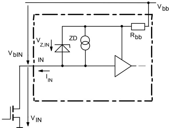
When the device is switched off ( $I_{IN} = 0$ ) the voltage between IN and GND reaches almost  $V_{bb}$ . Use a mechanical switch, a bipolar or MOS transistor with appropriate breakdown voltage as driver.
