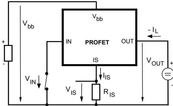
The device is specified for inverse load current operation ( $V_{OUT} > V_{bb} > 0V$ ). The current sense feature is not available during this kind of operation ( $I_S = 0$ ). With  $I_{IN} = 0$  (e.g. input open) only the intrinsic drain source diode is conducting resulting in considerably increased power dissipation. If the device is switched on ( $V_{IN} = 0$ ), this power dissipation is decreased to the much lower value  $R_{ON(INV)} \cdot I^2$  (specifications see page 4).
