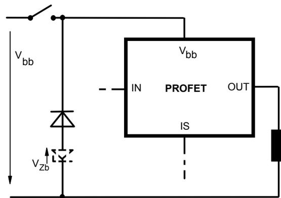
Note that there is no reverse battery protection when using a diode without additional Z-diode  $V_{ZL}$ ,  $V_{Zb}$ .
