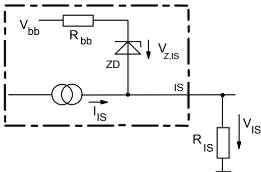
$V_{Z,IS} = 66\text{ V (typ.)}$ ,  $R_{IS} = 1\text{ k}\Omega$  nominal (or  $1\text{ k}\Omega / n$ , if  $n$  devices are connected in parallel).  $I_S = I_L / K_{iIs}$  can be only driven by the internal circuit as long as  $V_{out} - V_{IS} > 5\text{ V}$ . If you want to measure load currents up to  $I_{L(M)}$ ,  $R_{IS}$  should be less than  $\frac{V_{bb} - 5\text{ V}}{I_{L(M)} / K_{iIs}}$ .
