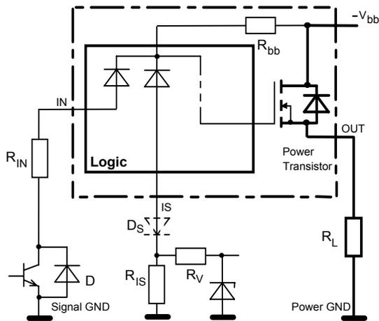
$R_V \geq 1 \text{ k}\Omega$ ,  $R_{IS} = 1 \text{ k}\Omega$  nominal. Add  $R_{IN}$  for reverse battery protection in applications with  $V_{bb}$  above  $16 \text{ V}^{19)}$ ; recommended value:  $\frac{1}{R_{IN}} + \frac{1}{R_{IS}} + \frac{1}{R_V} = \frac{0.1\text{A}}{|V_{bb}| - 12\text{V}}$  if  $D_S$  is not used (or  $\frac{1}{R_{IN}} = \frac{0.1\text{A}}{|V_{bb}| - 12\text{V}}$  if  $D_S$  is used).
