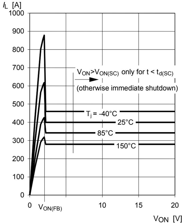
In case of  $V_{ON} > V_{ON(SC)}$  (typ. 6 V) the device will be switched off by internal short circuit detection.
