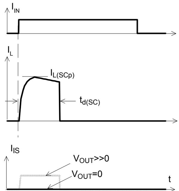
Shut down remains latched until next reset via input.
