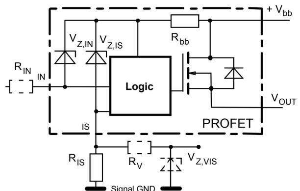
$R_{bb} = 120\ \Omega$  typ.,  $V_{Z,IN} = V_{Z,IS} = 66\text{ V typ.}$ ,  $R_{IS} = 1\text{ k}\Omega$  nominal. Note that when overvoltage exceeds  $71\text{ V typ.}$  a voltage above  $5\text{ V}$  can occur between IS and GND, if  $R_V$ ,  $V_{Z,IS}$  are not used.
