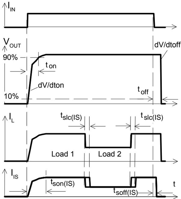
The sense signal is not valid during a settling time after turn-on/off and after change of load current.
