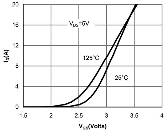
Figure 2: Transfer Characteristics
