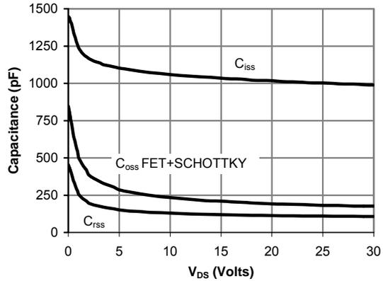
Figure 8: Capacitance Characteristics
