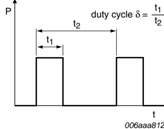
**Fig 13. Duty cycle definition**
