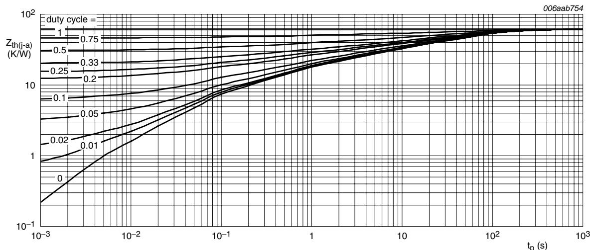
Ceramic PCB,  $\text{Al}_2\text{O}_3$ , standard footprint
