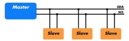
**Figure 1**: Sample I<sup>2</sup>C Implementation. – Regardless of how many slave units are attached to the I<sup>2</sup>C bus, there are only two signals connected to all of them. Consequently, there is additional overhead because an addressing mechanism is required for the master device to communicate with a specific slave device.
