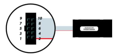
**Figure 6**: The Aardvark I<sup>2</sup>C/SPI Host Adapter in the upside down position. – Pin 1 is located in the lower left corner of the connector and Pin 10 is located in the upper right corner of the connector.
