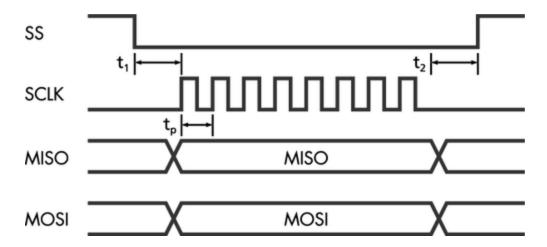
**Figure 7**: SPI Waveform – Three different times are of note:  $t_1$ , time from the assertion of SS# to the first clock cycle;  $t_2$ , time from the last clock cycle and the deassertion of SS#;  $t_p$ , clock period.
