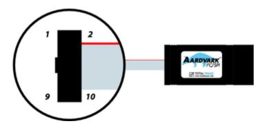
**Figure 5**: The Aardvark I<sup>2</sup>C/SPI Host Adapter in the upright position. – Pin 1 is located in the upper left corner of the connector and Pin 10 is located in the lower right corner of the connector.
