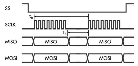
**Figure 8** : SPI Byte Timing  $-t_d$  is the setup time between SPI bytes and  $t_b$  is the total byte-to-byte time.
