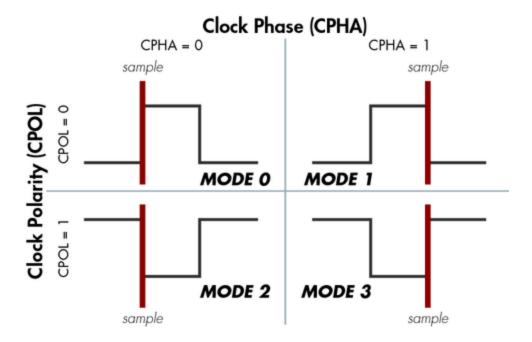
**Figure 4**: SPI Modes – The frame of the data exchange is described by two parameters, the clock polarity (CPOL) and the clock phase (CPHA). This diagram shows the four possible states for these parameters and the corresponding mode in SPI.
