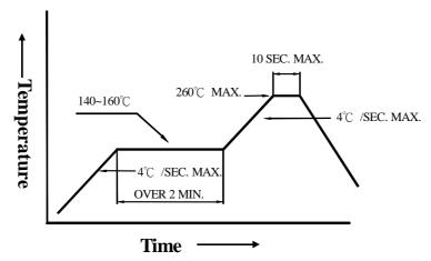
3. DIP soldering (Wave Soldering):
