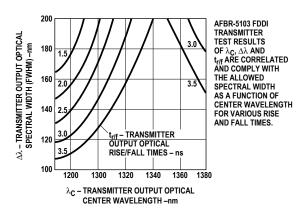
Figure 9. Transmitter Output Optical Spectral Width (FWHM) vs. Transmitter Output Optical Center Wavelength and Rise/Fall Times.
