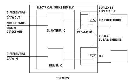
Figure 1a. ST Connector Block Diagram.
