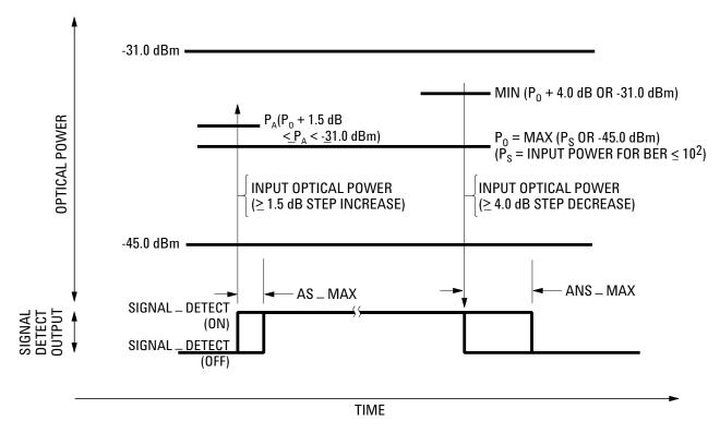
AS \_ MAX — MAXIMUM ACQUISITION TIME (SIGNAL). AS \_ MAX IS THE MAXIMUM SIGNAL \_ DETECT ASSERTION TIME FOR THE STATION. AS \_ MAX SHALL NOT EXCEED 100.0  $\mu$ s. THE DEFAULT VALUE OF AS \_ MAX IS 100.0  $\mu$ s.
