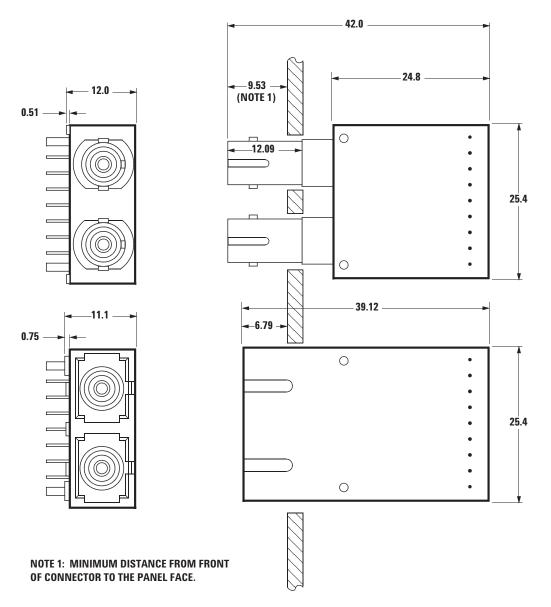
Figure 8a. Recommended Common Mechanical Layout for SC and ST 1 x 9 Connectored Transceivers.
