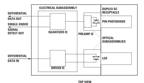
Figure 1. SC Connector Block Diagram.
