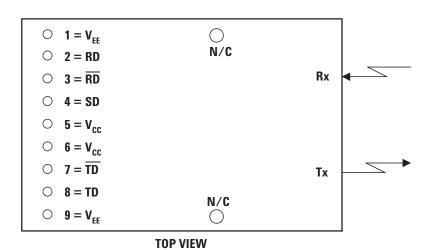
Figure 3. Pin Out Diagram.
